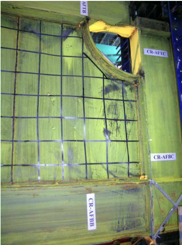
Figure 9: Infill panel and RBS yielding (Specimen CR: Cycle 19, \gamma = 1.5\% \approx 5\delta )
